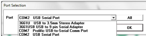
The black software cable connects the meter to the computer data port. Select the Com Port that is assigned to the computer data port. See "Identifying the Correct Com Port" (p. 6) for instructions on how to determine which port to select.
