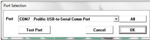
The computer **Communications Port** to which the PC-3.5mm serial cable is connected
